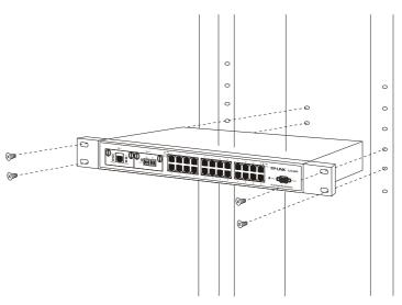
Figure 3-1 Rack Installation
